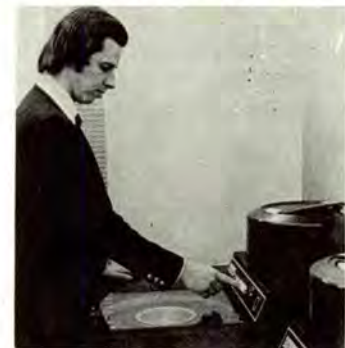
Jack Pickett, one of the Center's computer operators, starts a disc file into operation. These discs are the "file cabinets" for all computerized information. Docket information on thousands of cases from many districts can be stored on the two discs shown here.
